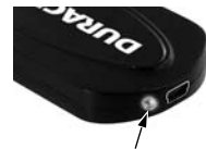
3.3 - 3.4: A red light here on the Universal Battery indicates that the Universal Battery is being charged. When the battery is fully charged, this light becomes green.
